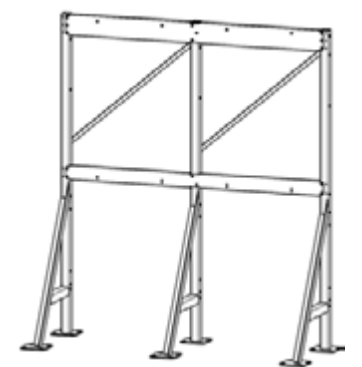
R-138 : 2 boiler rack only
